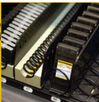
Expansion module spiral machine: Multi-supplier capability with drawers for restricted access when stocking.
